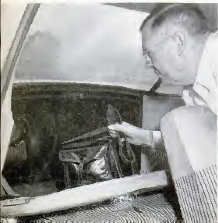
Owners object to lack of outside opening in trunk. To load it, you have to pull down the rear-seat back
